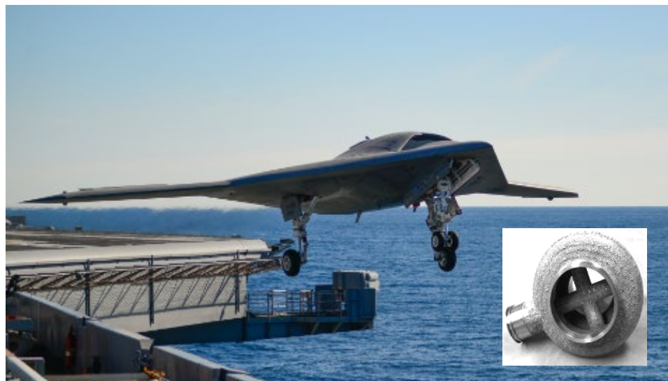
1 st Flight of an AM PBF Titanium Component on a DoD Platform
